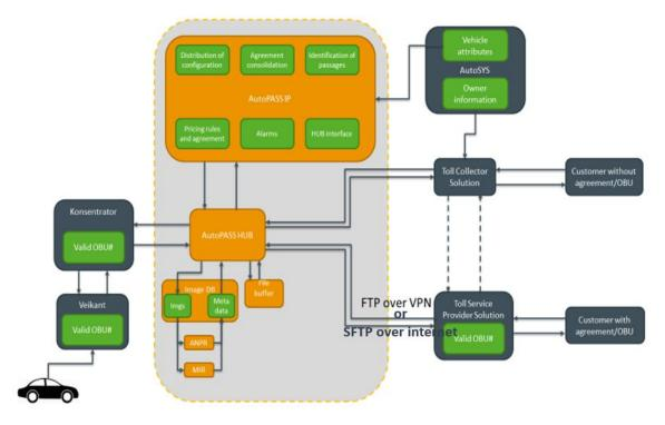
Figure 1 - AutoPASS actors/systems and data exchange interfaces subject to testing
